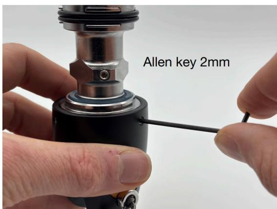
In this case, fully remove the screw, clean any glue residue, and reinsert it with a drop of Loctite 243
