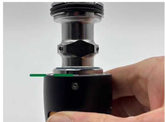
If the end-stop support (A) is not screwed in (threads are visible), contact Karver customer service (SAV) for the reassembly procedure.
