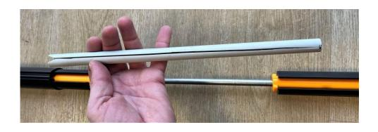
Using the notch made in the split plastic tube, fit the tube around the forestay between the 2 junctions.
