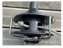
Lights at the bottom of the drum allows to fix a single line with simple stop knot.
