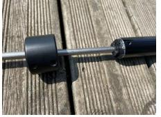
Insert the junction assembly / bearings fully in the profile.
