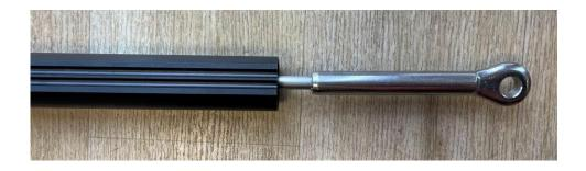
Swaged end fitting remains out of the foil (standard)
