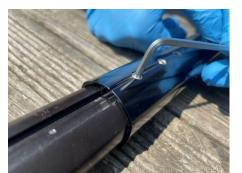
Collect the junction screws and the Torx key from the package, screw with a maximum torque of 5N.m, the screws must not.
