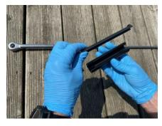
Insert the foil top endstop first. Take the top junction and insert a half bearing into it.
