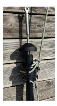
Hook a halyard onto the swivel and pull it up against the foil top endstop.
