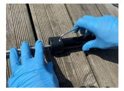
Insert the upper foil top endstop and screw the M8 stainless steel grub screw (K) into the hole just made in the upper profile.
