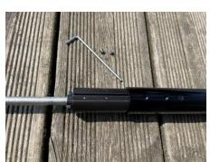
The junction equipped with the bearings is inserted only halfway (up to a screw acting as a track endstop)
