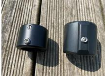
2 Types of profile top endstops exist, in both cases the stainless steel screw is oriented towards the bottom of the reefing headsail furler.
