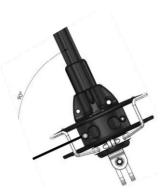
The position of the first return block must allow entry of the rope into the drum of the furler at an angle of 90° in relation to the profiles.
