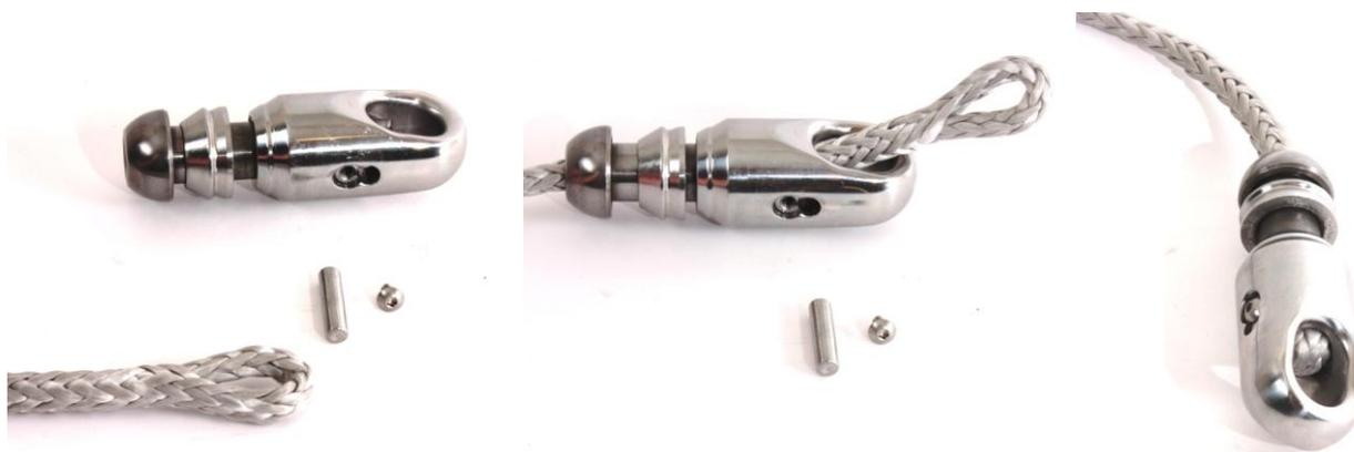
Splice your halyard and fit it into the male part (G). The splice should feature a max diameter of 9.5mm.
